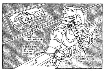
No-daily-maintenance undercarriage saves you time and work. Track rollers, carrier rollers and idlers are Lifetime Lubricated, sealed with Duo-Cone® Floating Ring Seals to keep in lubricant... keep out abrasives. Standard hydraulic track adjusters keep proper tension with occasional adjustment with a grease gun.
