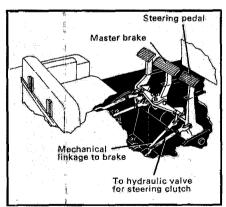
Three pedals do the work . . . for turns and stops. Push the right or left pedal halfway down to release the steering clutch for a slow turn . . . all the way down to brake for a sharp turn. The center pedal also brakes both tracks without releasing the clutches . . . and locks down as a parking brake. The steering clutches are oil-cooled, heavyduty multiple discs. The brakes are oil-cooled contracting bands. Both are a single unit for easy lift-out and servicing.
