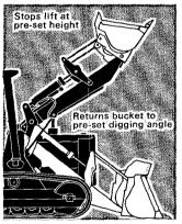
Automatic bucket controls let you concentrate on maneuvering the machine . . . rather than positioning the bucket. Move lift lever into detent position, then let go - the loaded bucket rises to a preset dumping height and automatically stops when the lever kicks out. A similar arrangement on the tilt lever returns the empty bucket to a pre-set digging angle before the loader re-enters the pile or bank. Both controls can be adjusted and manually overridden.
